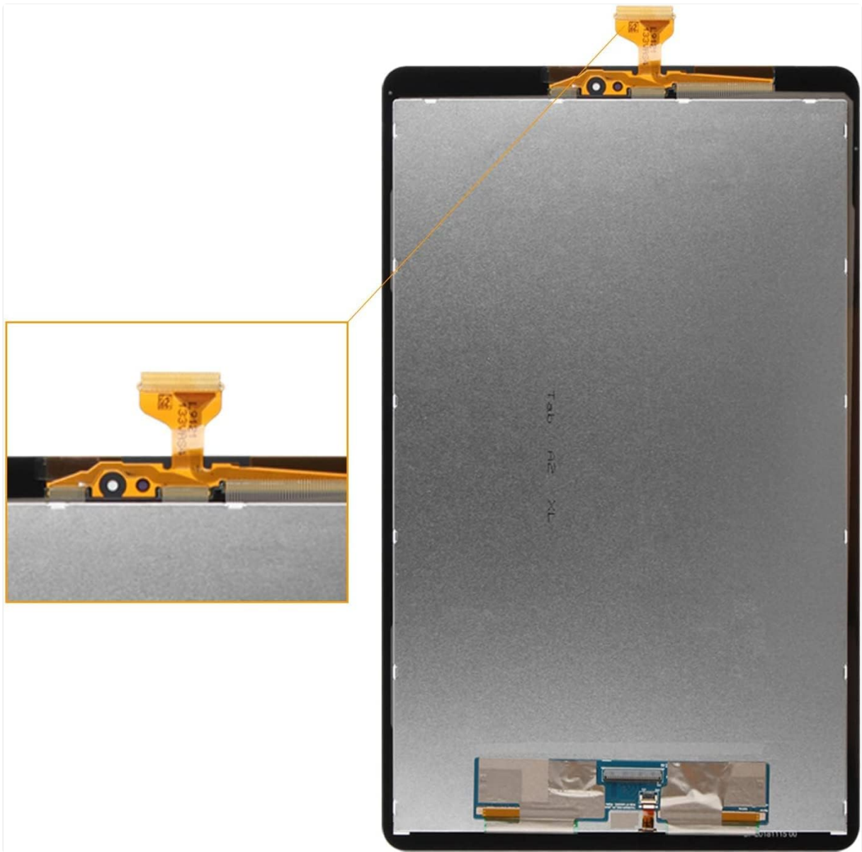
Image: Rear view of the replacement screen, highlighting the flex cables and connectors that need careful handling during installation.
