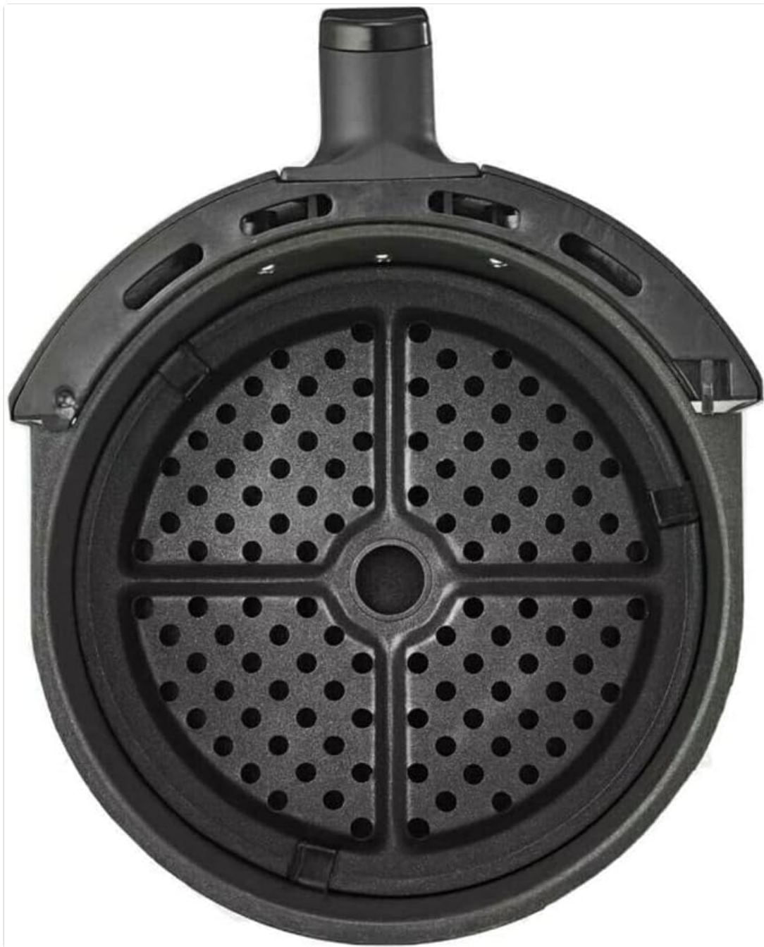
Figure 4: An inside view of the air fryer's crisping tray, featuring a perforated design to allow hot air to circulate evenly around food for optimal crisping.
