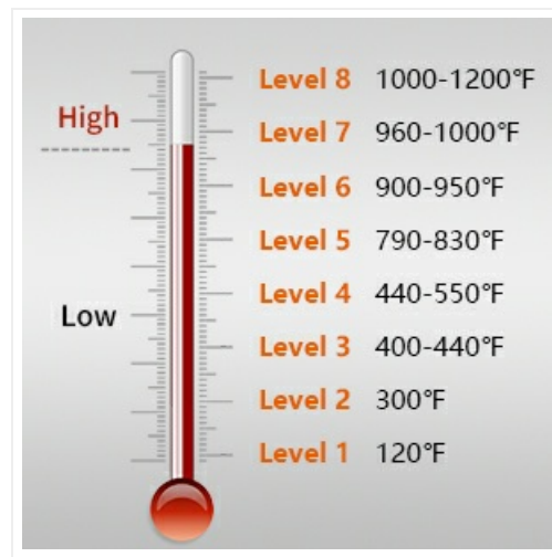
Figure 5.3: Approximate temperature levels corresponding to the dial settings.
