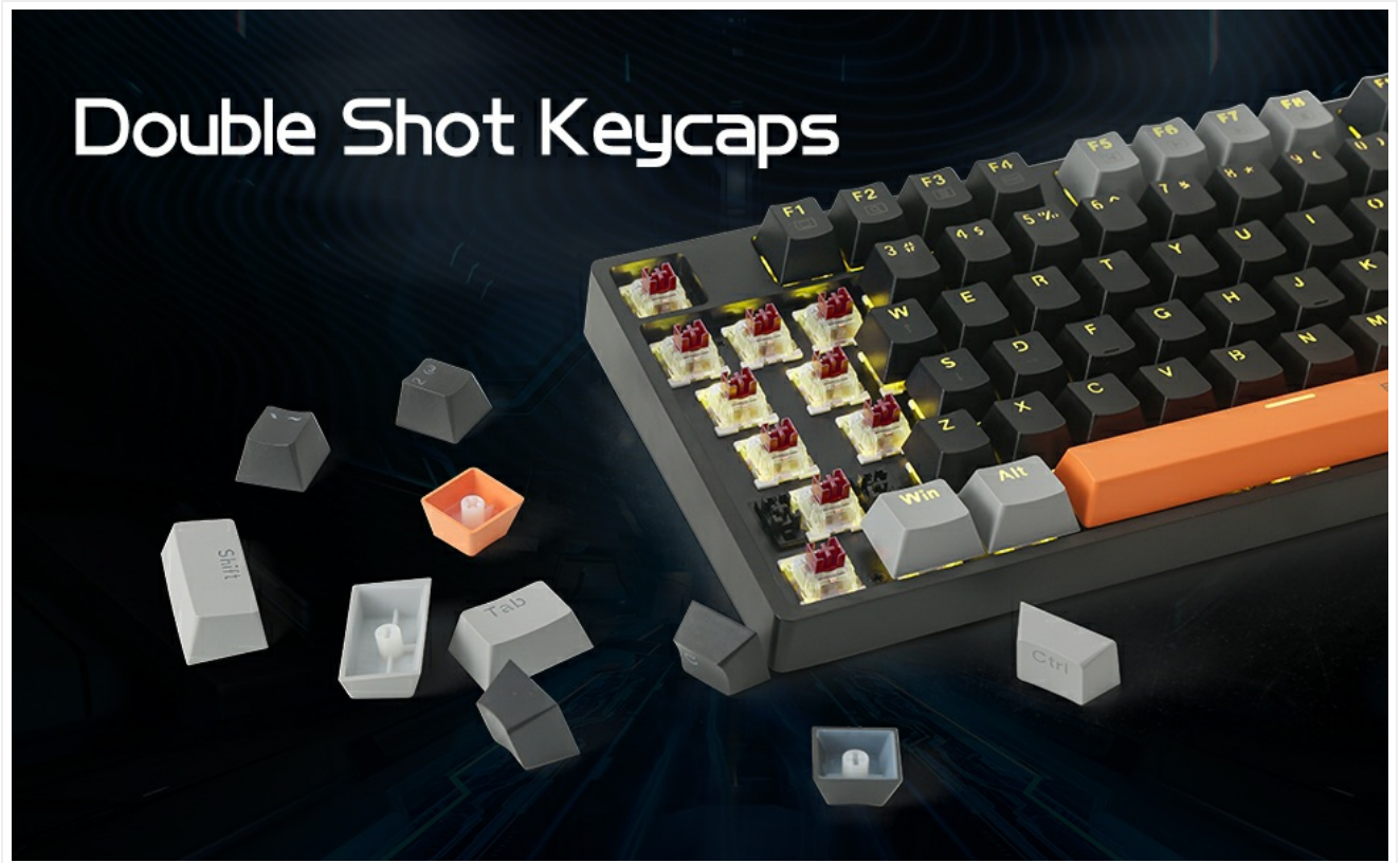
Figure 4: Detail of hot-swappable switches and double shot keycaps.
