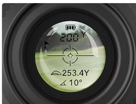
Figure 7: View through the rangefinder showing slope compensation.
