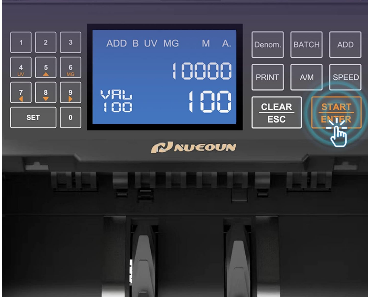
Figure 4.2: Control Panel and LED Display
