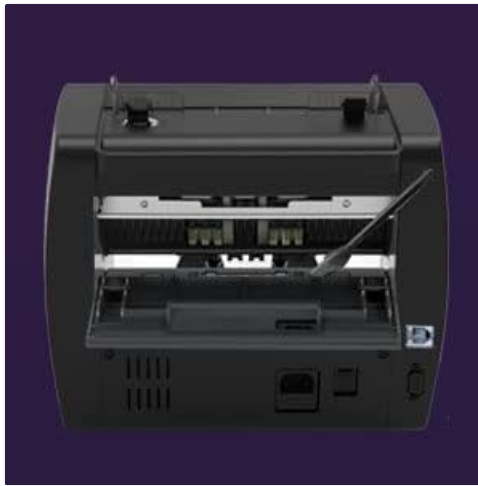
Figure 7.1.1: Open Passage for Cleaning
