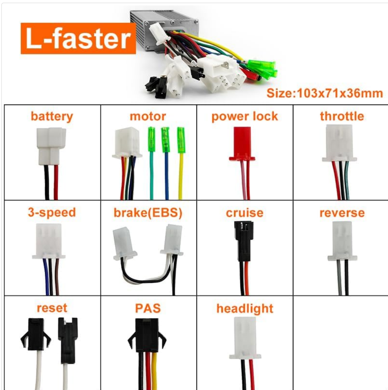
Figure 4.1: Detailed view of individual wiring connectors. This image helps identify the specific plugs for battery, motor, power lock, throttle, 3-speed, brake (EBS), cruise, reverse, reset, PAS, and headlight connections.
