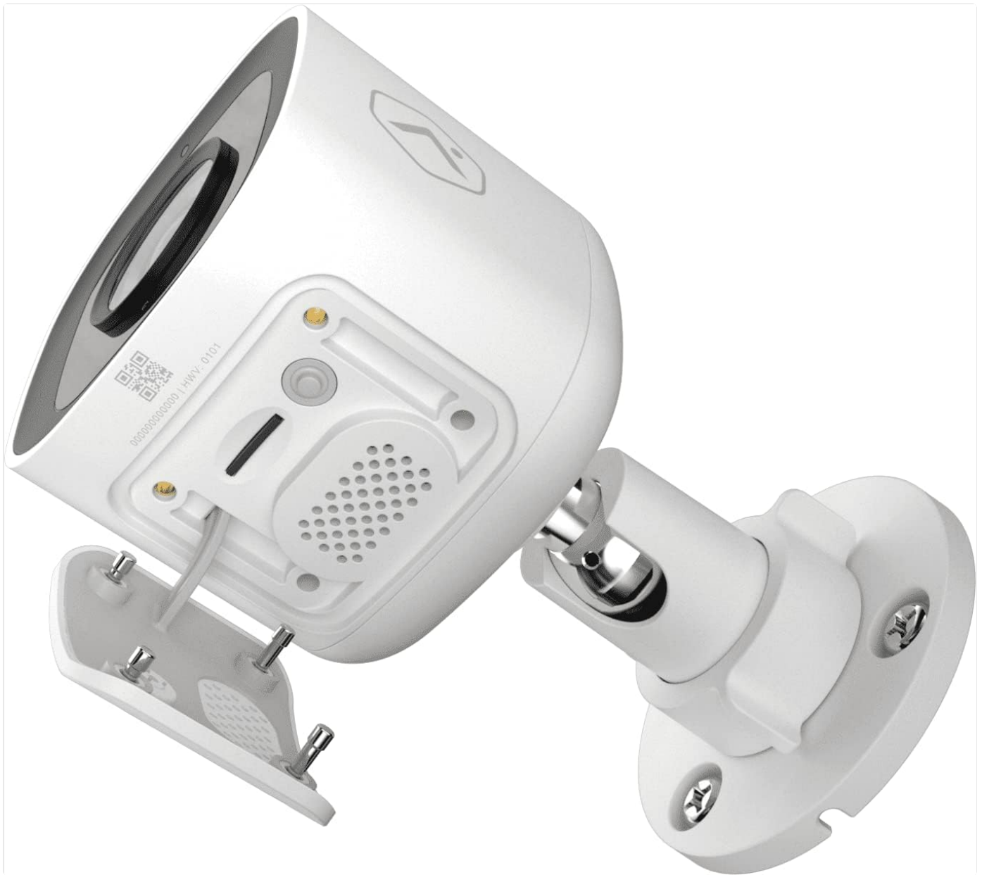
Figure 5: Bottom view of the camera showing the access panel for the MicroSD card slot.
