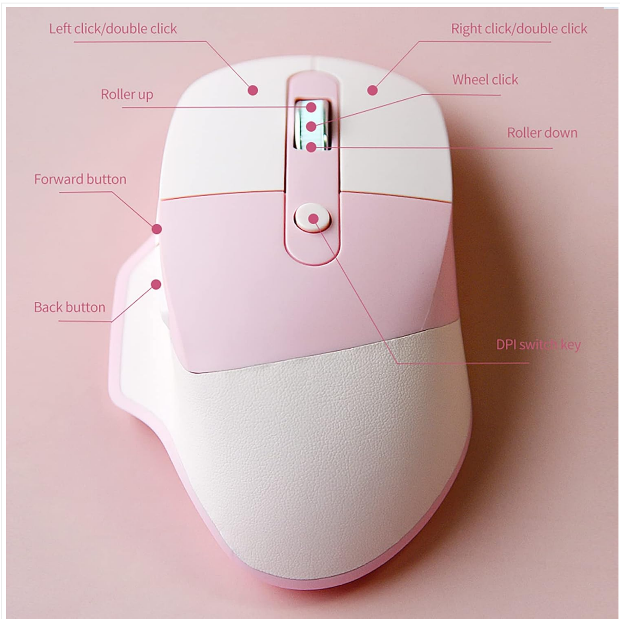
Image: Diagram illustrating the various buttons and their functions on the mouse.
