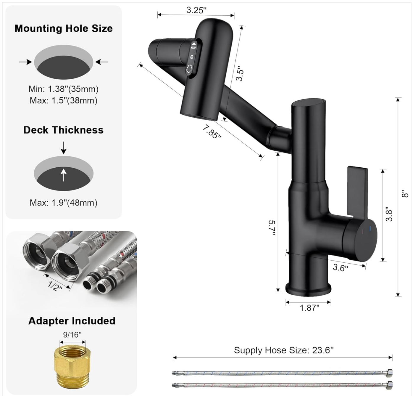
Image 4.1: Mounting hole and deck thickness specifications.
