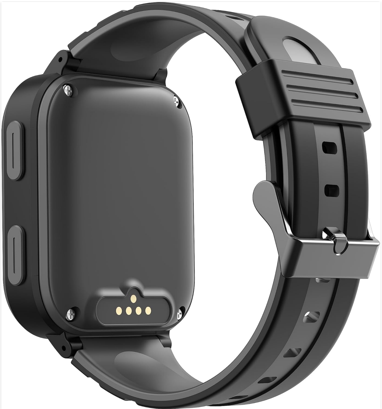
Image: Back view of the SW2, showing the magnetic charging pins.
