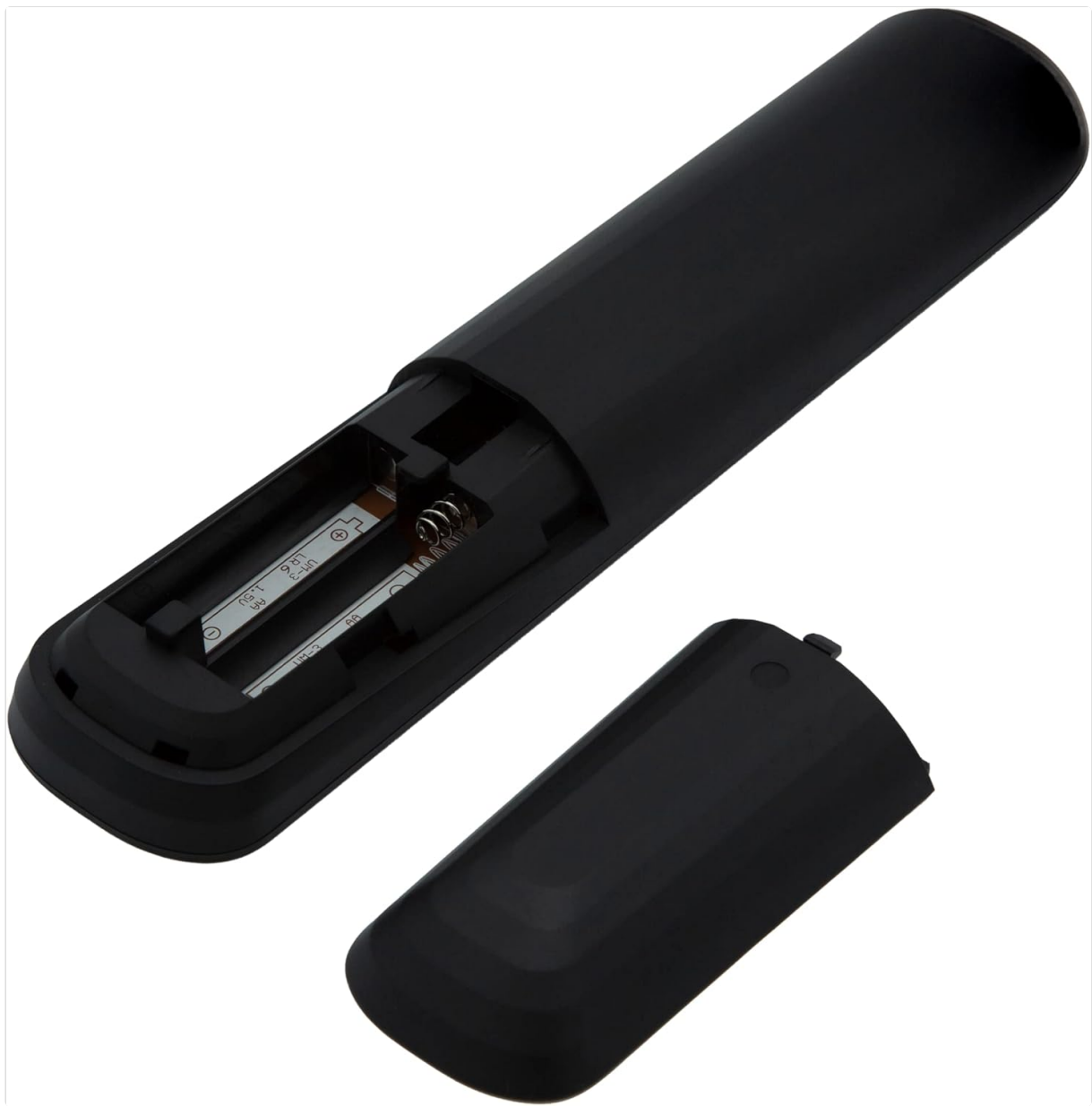
Image: The back of the BuzzTV IR-200 remote control with the battery compartment open, showing where to insert two AAA batteries.
