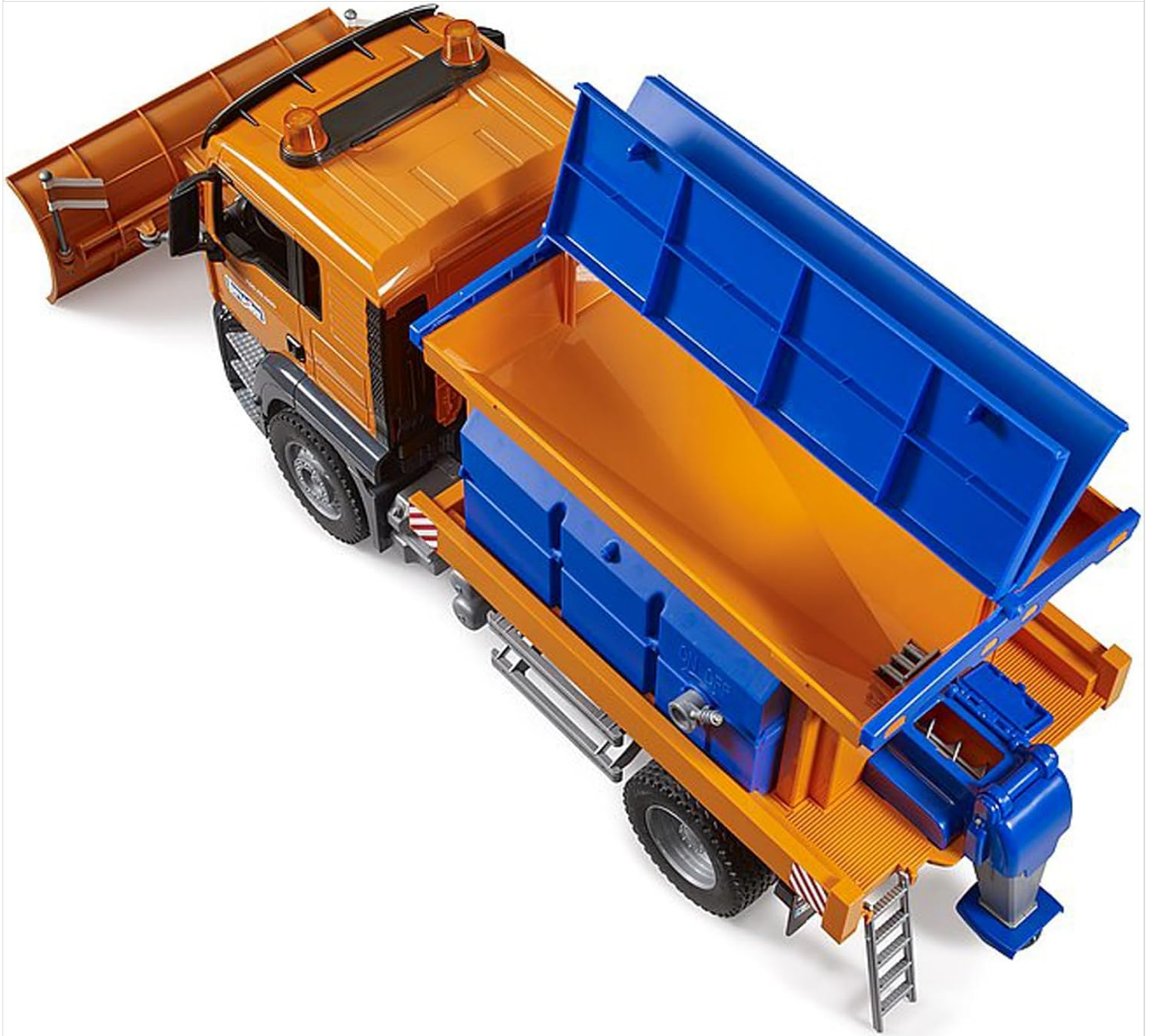
Image 4.3: The spreader unit with its top cover open, showing the fillable tank.
