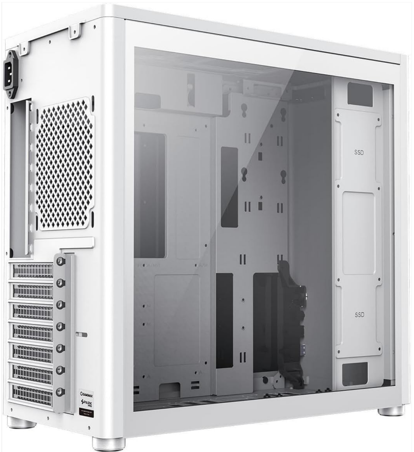
Figure 3.1: Rear view of the PC case, highlighting the power supply unit (PSU) mounting area and expansion slots.
