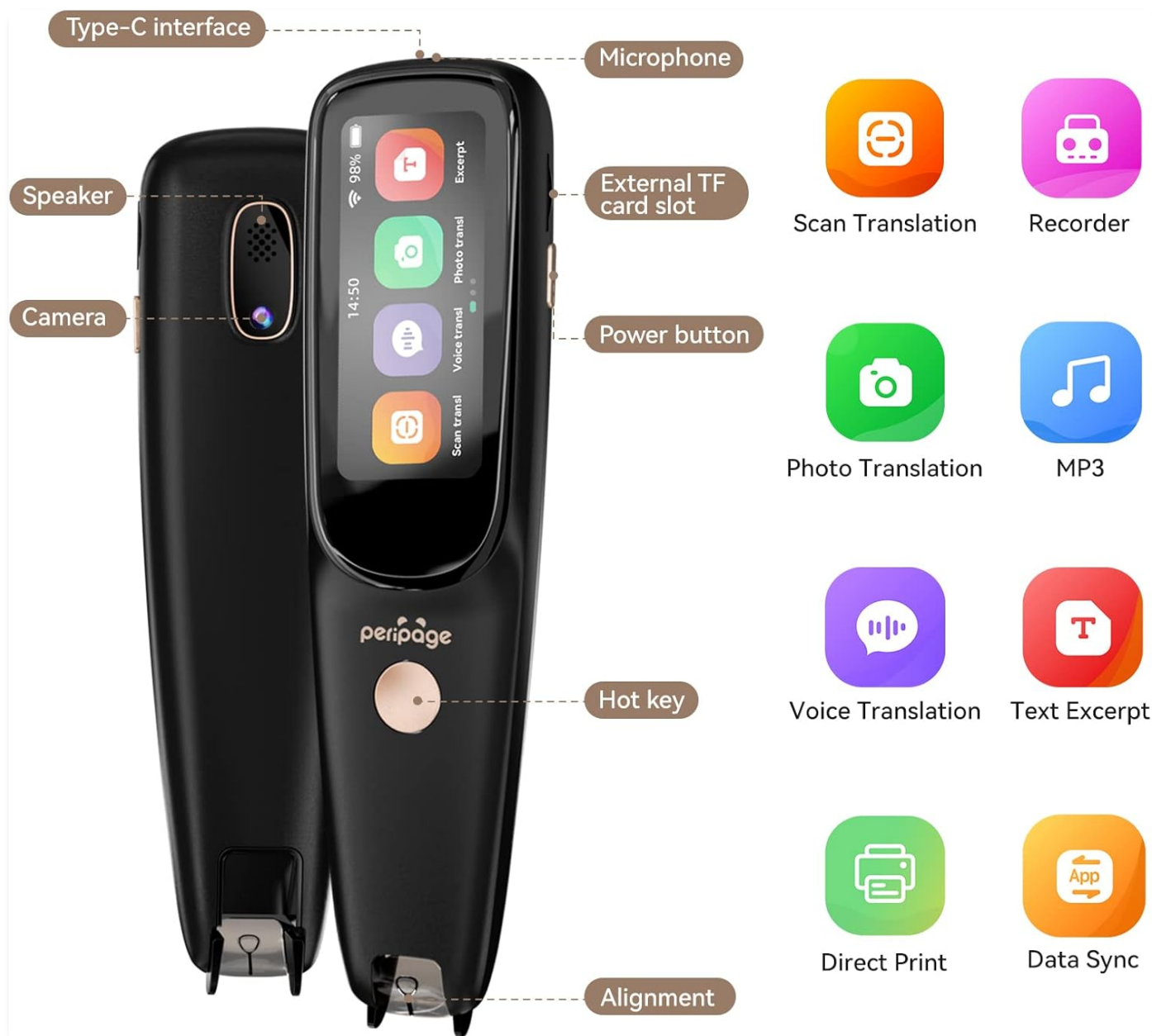
Figure 2: Components of the PeriPage D2s Scanning Pen. This diagram illustrates the physical features and on-screen functions of the device, including ports, buttons, and application icons.
