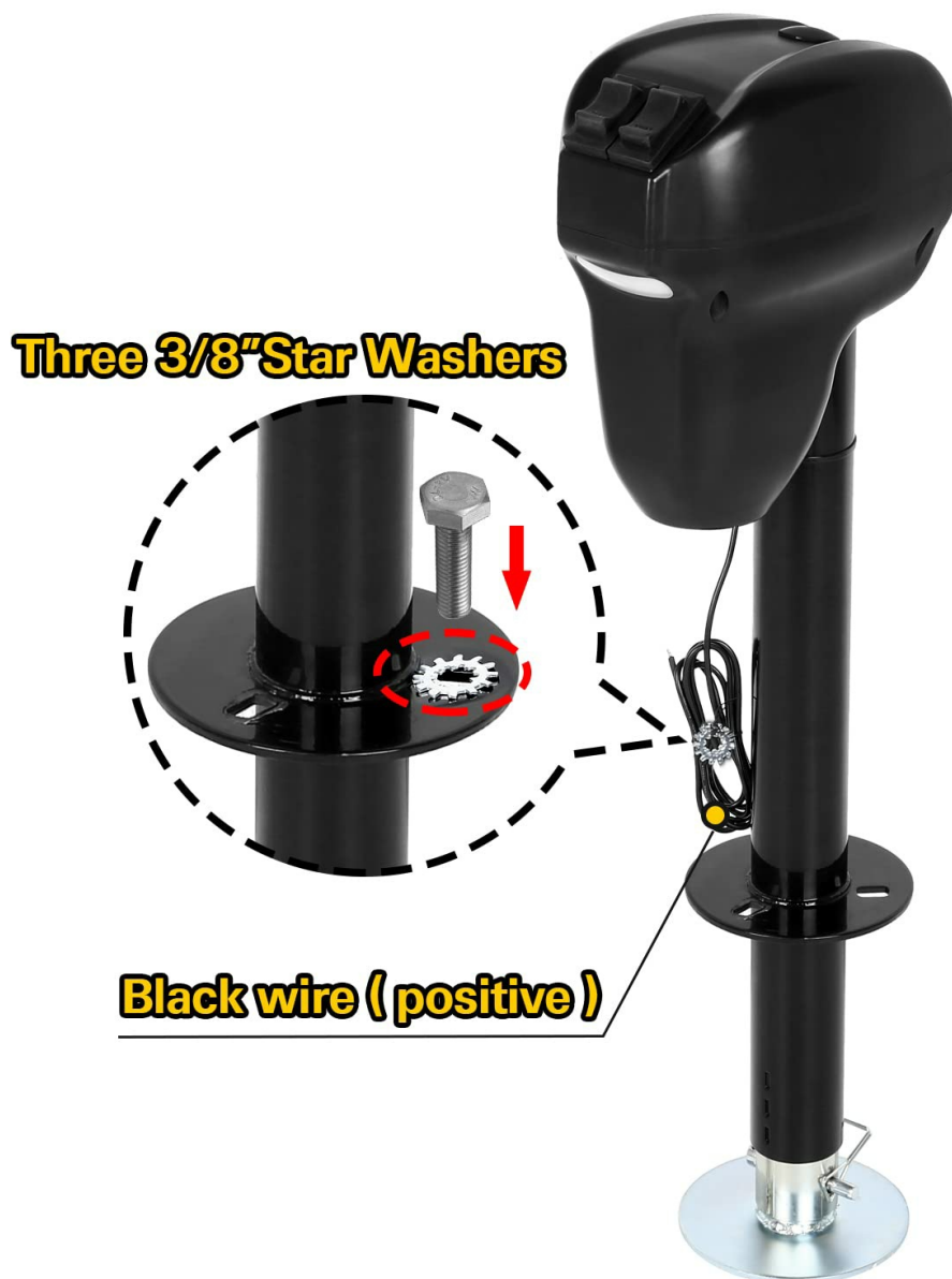
Figure 4: Close-up detail showing the placement of three 3/8" star washers for proper grounding and the connection point for the black positive wire.
