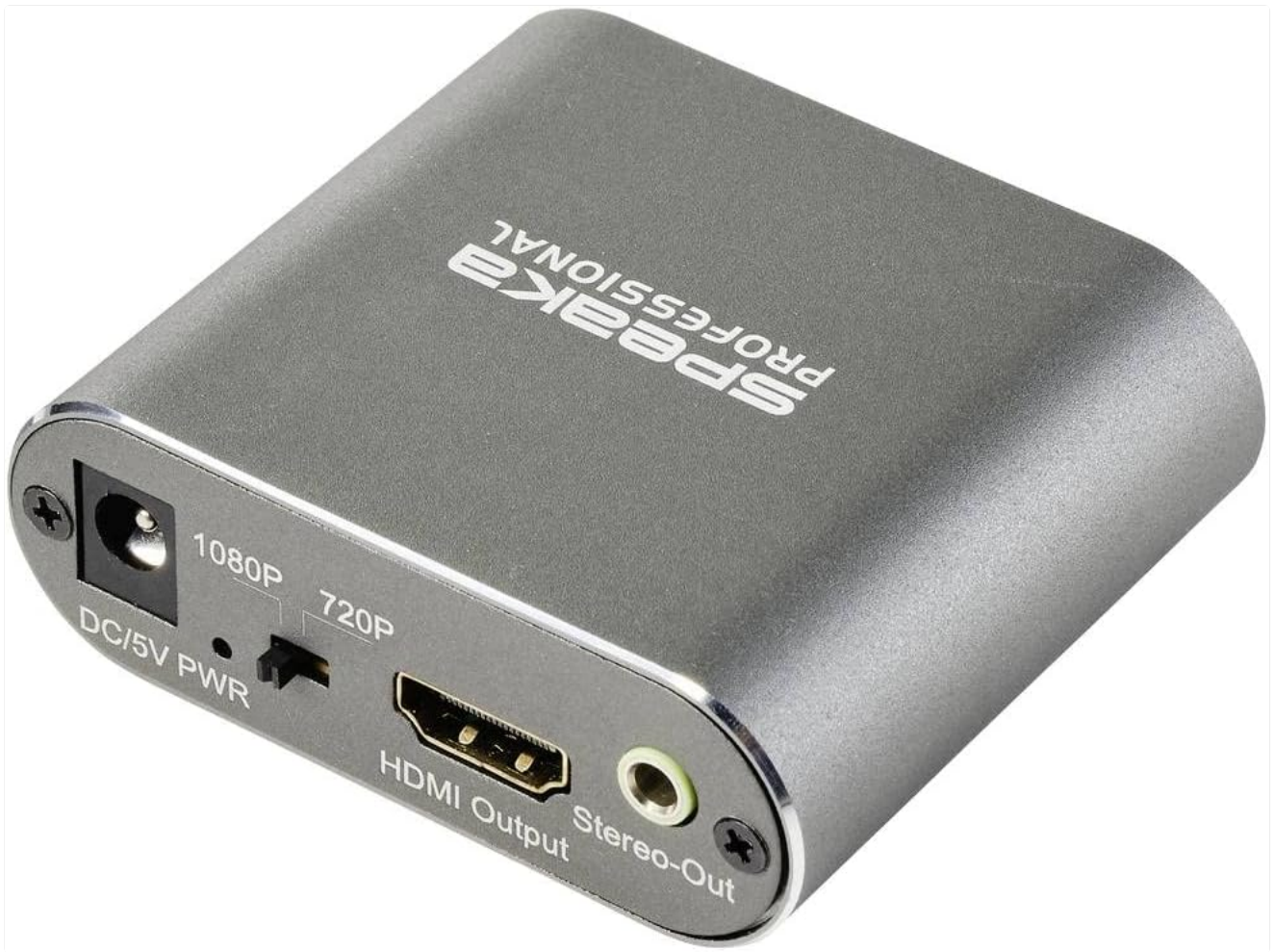
Image: Close-up of the SpeaKa Professional SP-SHC-200 showing the resolution switch between 1080P and 720P.
