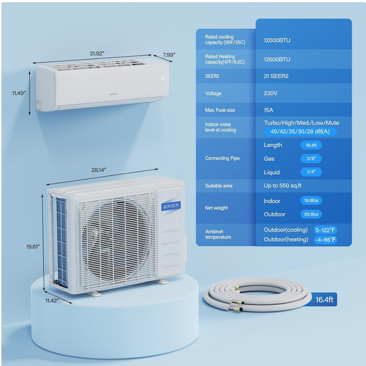
Image: A detailed diagram providing the dimensions of both the indoor and outdoor units of the ROVSUN mini split system, alongside a table listing key performance specifications such as BTU, SEER2, voltage, noise level, and suitable area coverage.
