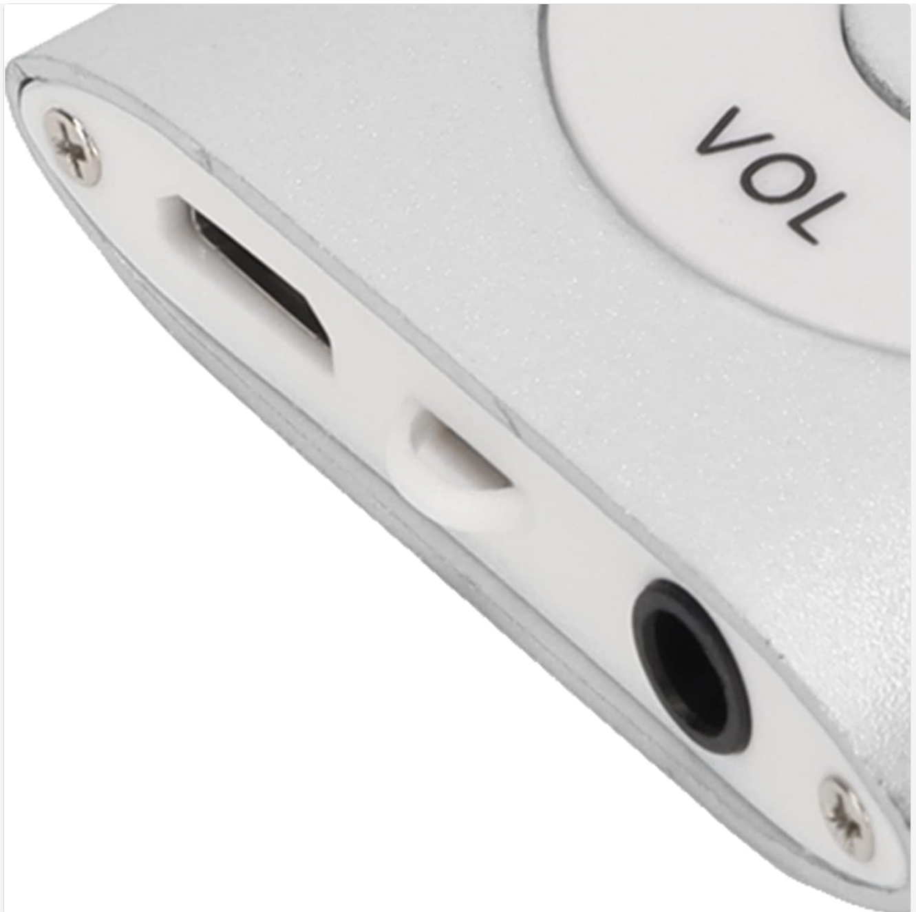
Image: Detailed view of the bottom of the MP3 player, showing the USB port, headphone jack, and microSD card slot.
