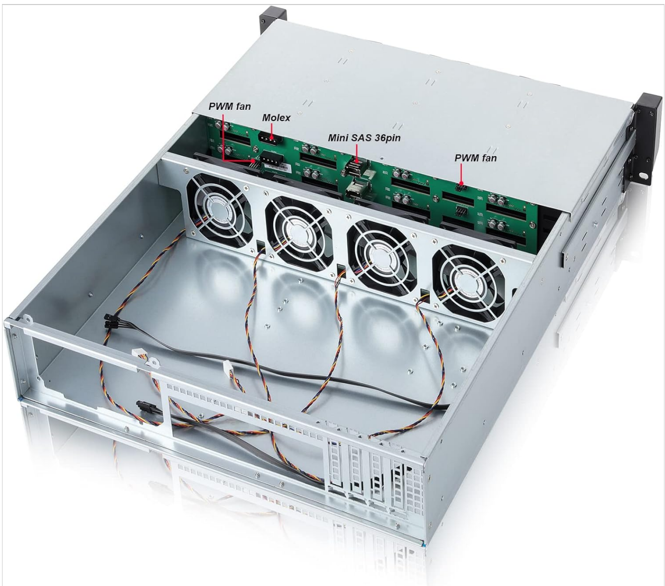
Figure 5: Internal view showing cooling fans and backplane.
