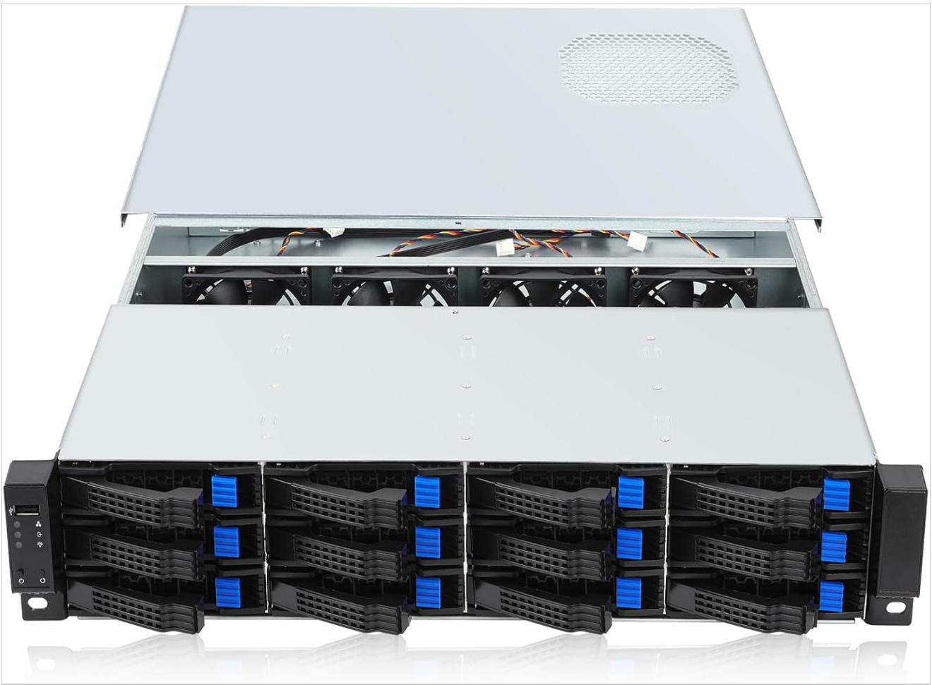
Figure 1: RackChoice 2U Rackmount Server Chassis with top cover removed.
