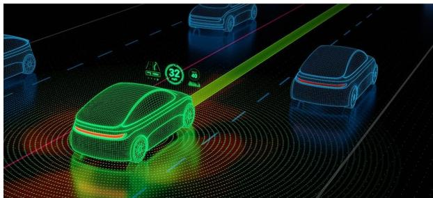
An illustrative image showing a car on a road with digital overlays indicating ADAS warnings such as lane departure and forward collision alerts.
