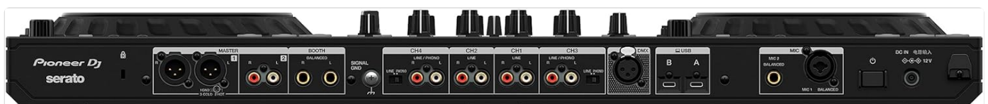
Figure 3: Rear panel of the DDJ-FLX10, displaying master outputs (XLR, RCA), booth output, channel inputs (Line/Phono), microphone inputs, and USB ports for computer connection.
