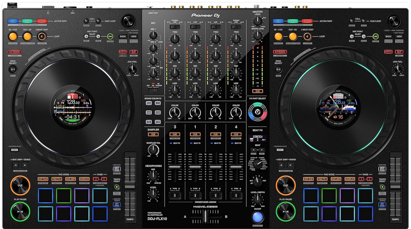
Figure 1: Top view of the DDJ-FLX10 controller, showcasing its layout with two large jog wheels, a central mixer section, and performance pads.
