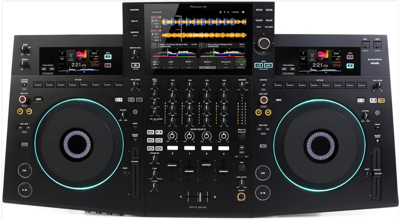
Image: Front view of the Pioneer DJ OPUS-QUAD 4-channel DJ System, highlighting the central 10.1-inch touchscreen display and the two large jog wheels with illuminated rings.
