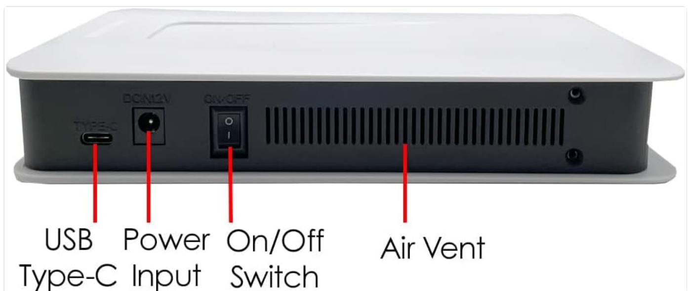
Figure 3.2: Rear Panel Connections. This image labels the USB Type-C port, power input, on/off switch, and air vents on the back of the hard drive.
