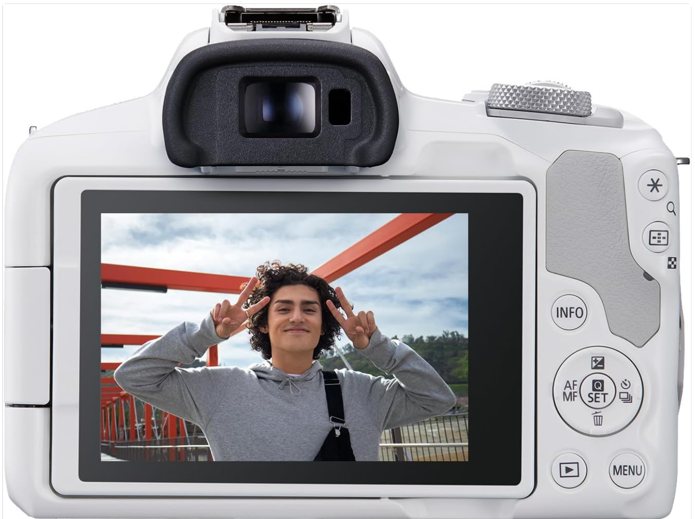
Image: Rear view of the Canon EOS R50 camera, highlighting the electronic viewfinder, LCD touchscreen, and various control buttons such as INFO, AF/MF, SET, and MENU.
