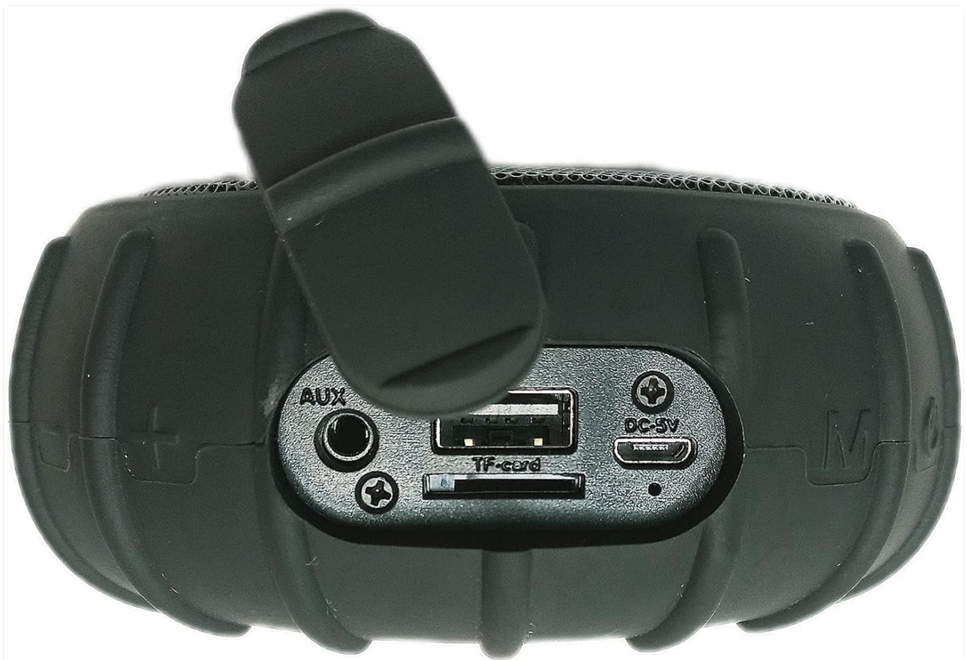
Image 4.1: Rear view of the speaker, highlighting the AUX, USB, DC-5V charging, and TF-card ports.
