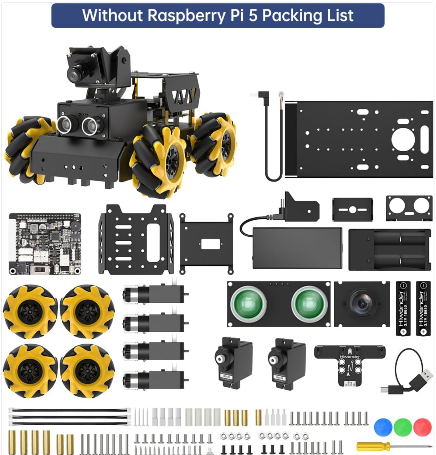
Image: All components included in the TurboPi Robot Car kit, excluding the Raspberry Pi board.
