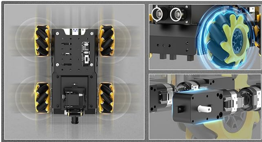
Image: Detailed view of the Mecanum wheels and motor assembly, enabling 360-degree movement.
