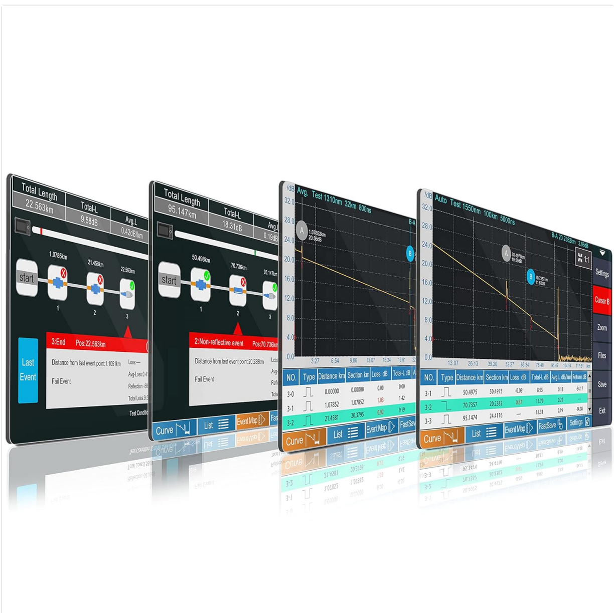
Figure 6.2: Examples of OTDR curve analysis, showing total length, total loss, average loss, and detailed event lists for different fiber segments.
