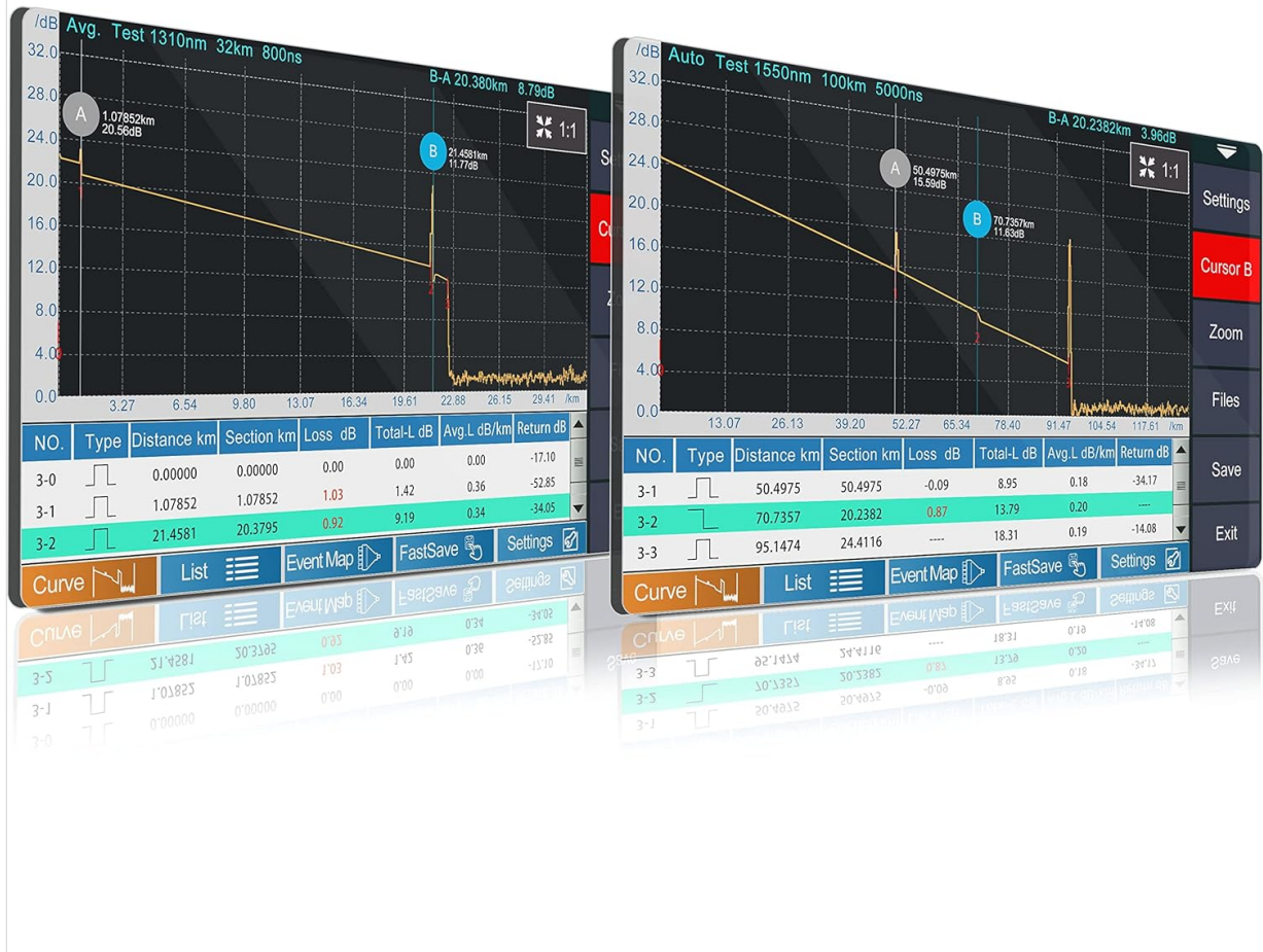
Figure 6.3: A comparison of OTDR test curves at 1310nm and 1550nm, illustrating how different wavelengths can reveal distinct characteristics of the fiber link.
