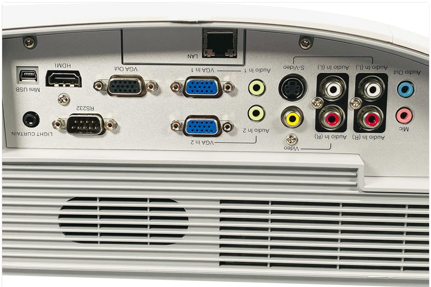
Figure 2: Rear panel of the Boxlight P8 WX35NXT projector, detailing the various input and output ports. From left to right, ports include Mini USB, HDMI, RS232, VGA Out, VGA In (x2), LAN, S-Video, Composite Video (RCA), Audio In (L/R), Audio Out, and Microphone input.
