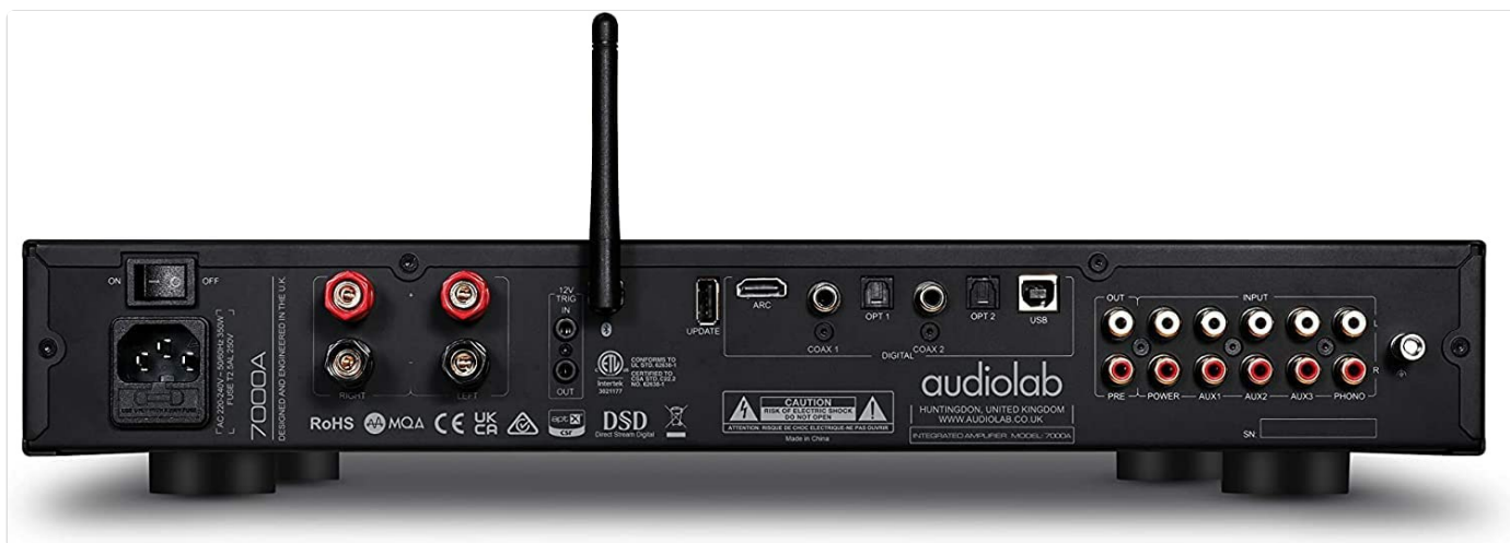
Figure 3: Rear panel of the Audiolab 7000A, showing various input and output terminals including power inlet, speaker terminals, analog RCA inputs, digital coaxial and optical inputs, HDMI ARC, USB-B, and a Bluetooth antenna.
