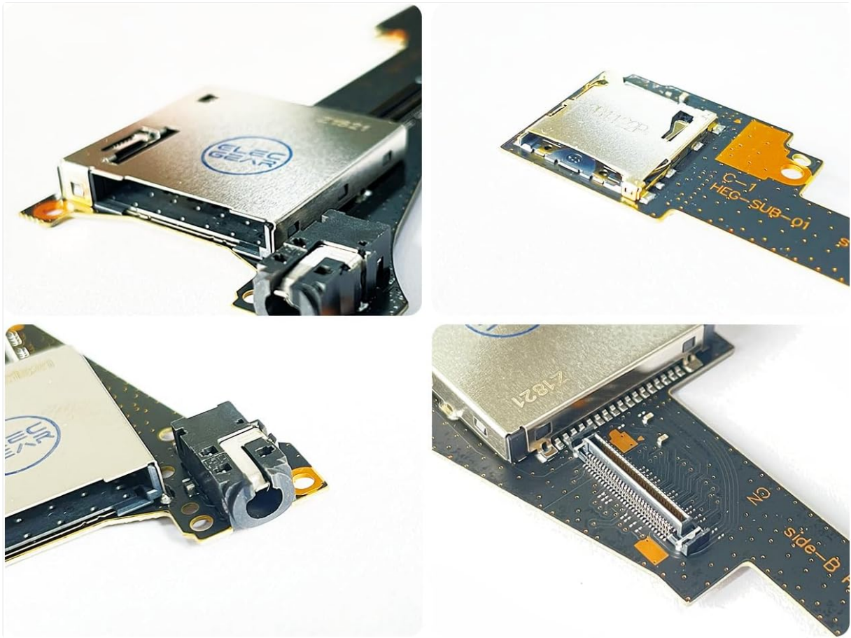
Image 1.1: Detailed view of the ElecGear replacement card reader module, highlighting the game card slot, Micro SD card slot, and the integrated 3.5mm headphone jack.
