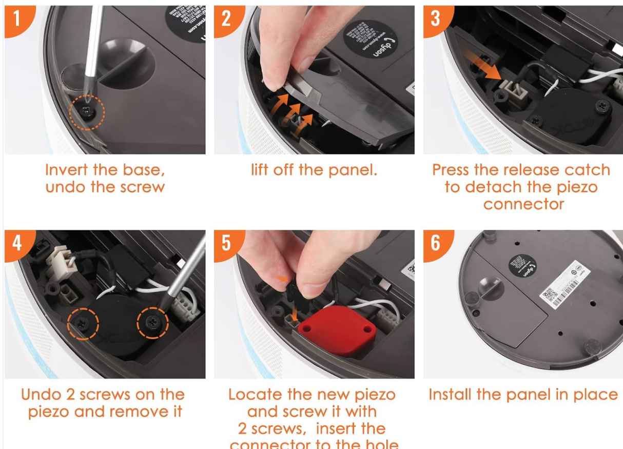
Figure 4: Visual guide detailing the six steps for piezo replacement.
