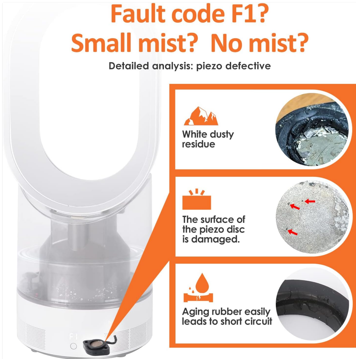
Figure 6: Visual representation of humidifier issues such as F1 fault code, small mist, or no mist, often caused by a defective piezo.
