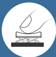
Figure 5.5: The concave keycaps are specifically designed to conform to the shape of your fingertips, enhancing typing comfort.
