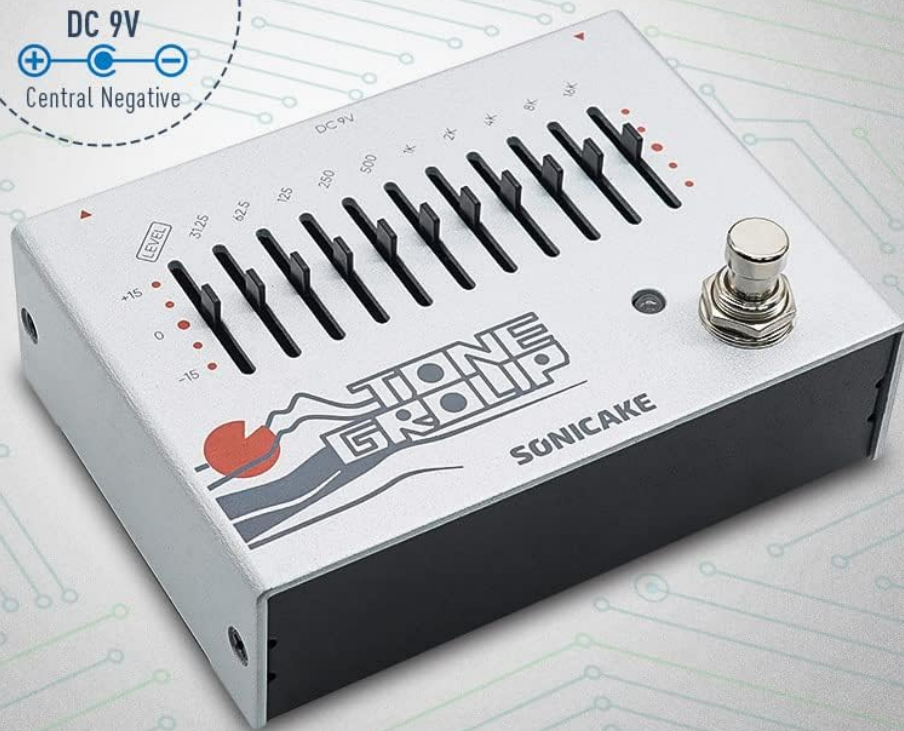
Image: An angled view of the EQ Equalizer pedal, highlighting the DC 9V power input and its central negative polarity requirement.
