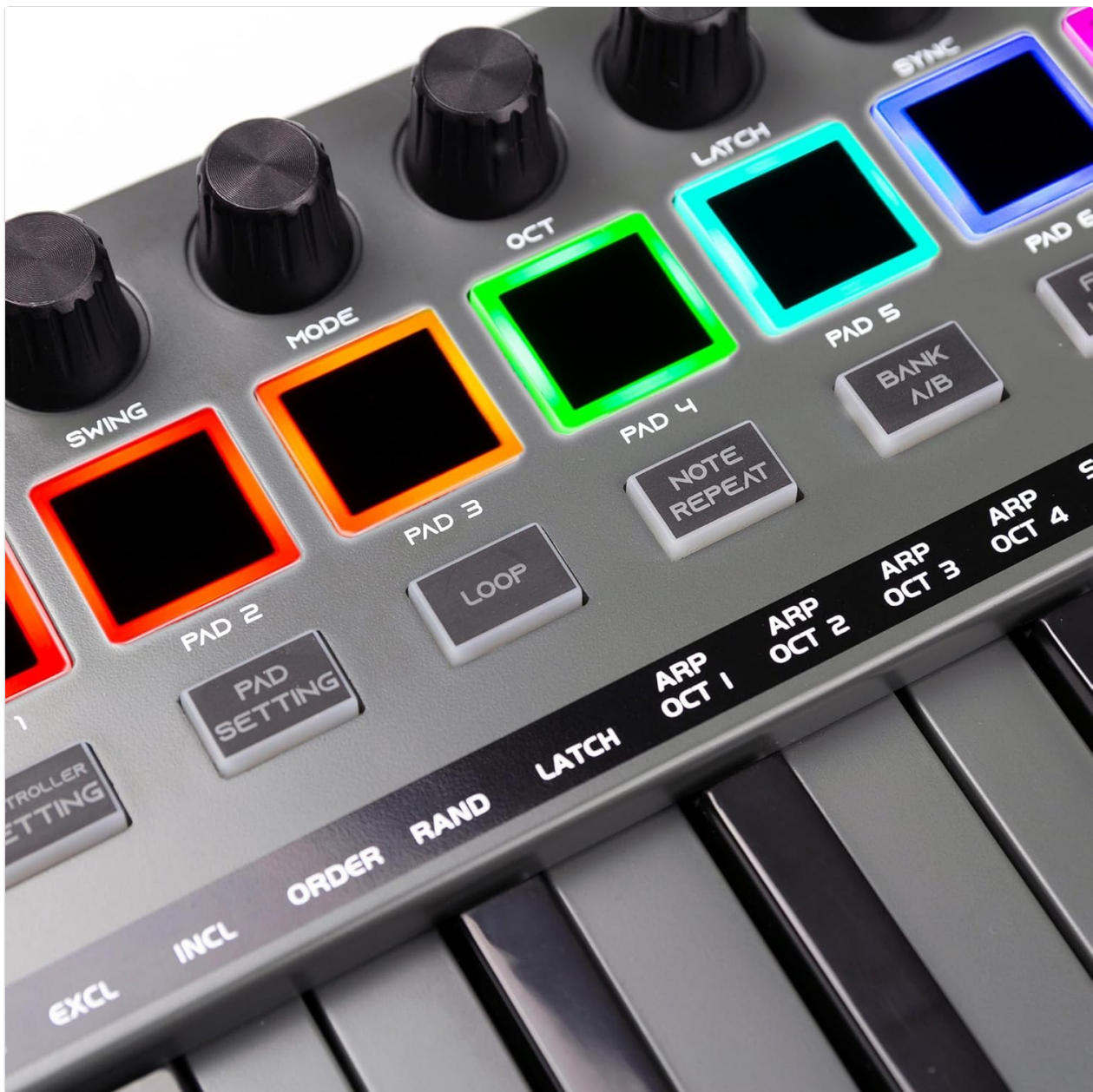
Figure 2.4: Close-up of the 8 backlit velocity-sensitive drum pads and 8 assignable control knobs.
