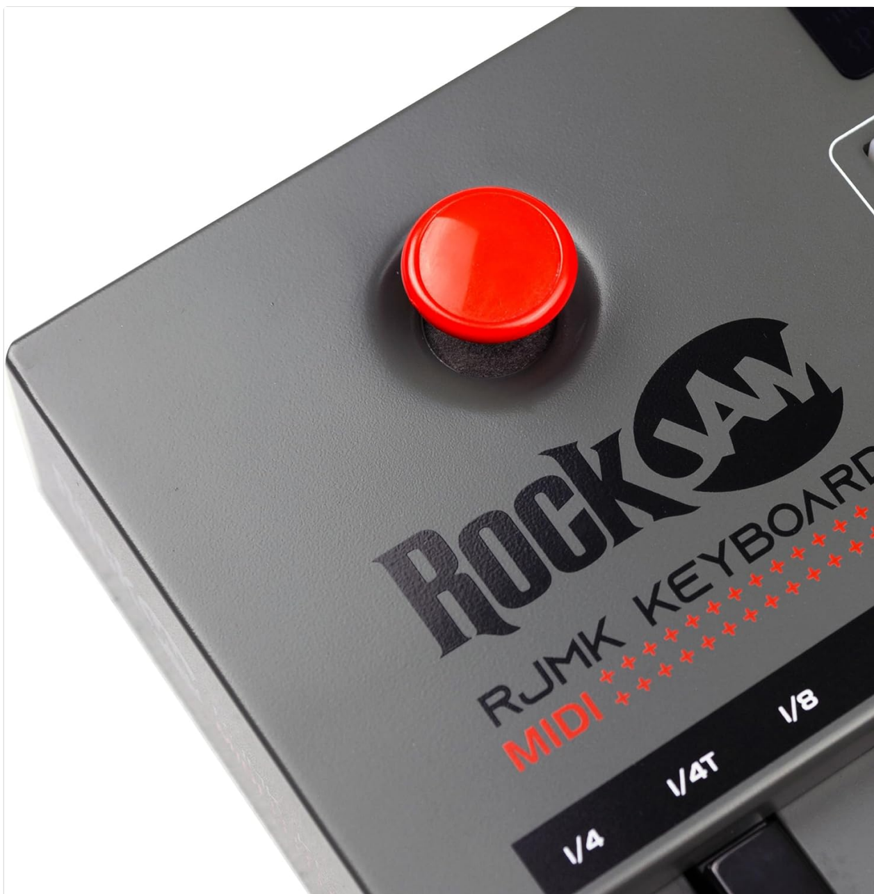
Figure 2.5: Detail of the omni-directional joystick for pitch and modulation control.
