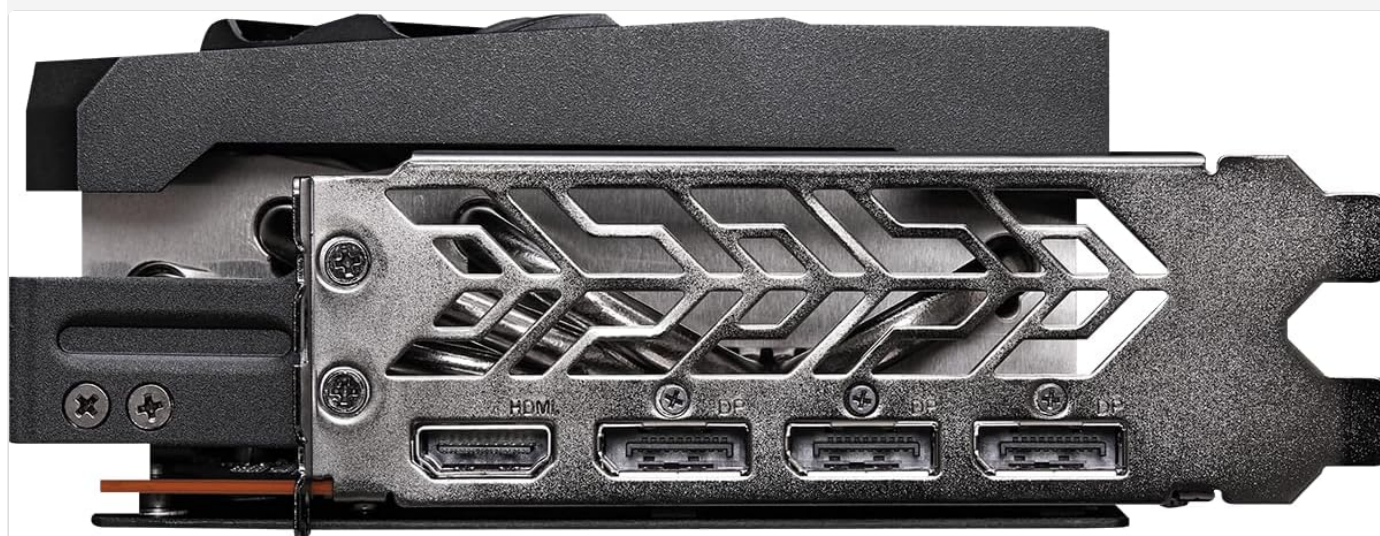
Figure 4: Rear view of the graphics card, detailing the three DisplayPort 2.1 and one HDMI 2.1 output ports for display connectivity.
