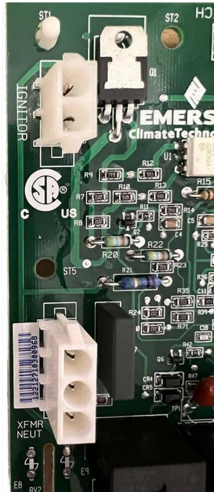
A close-up shot of the Hayward HDXFICBRD001 Ignition Control Board, specifically showing the 'IGNITOR' connection point (ST1). This is where the ignitor component of the gas heater connects to receive the signal for initiating combustion.
