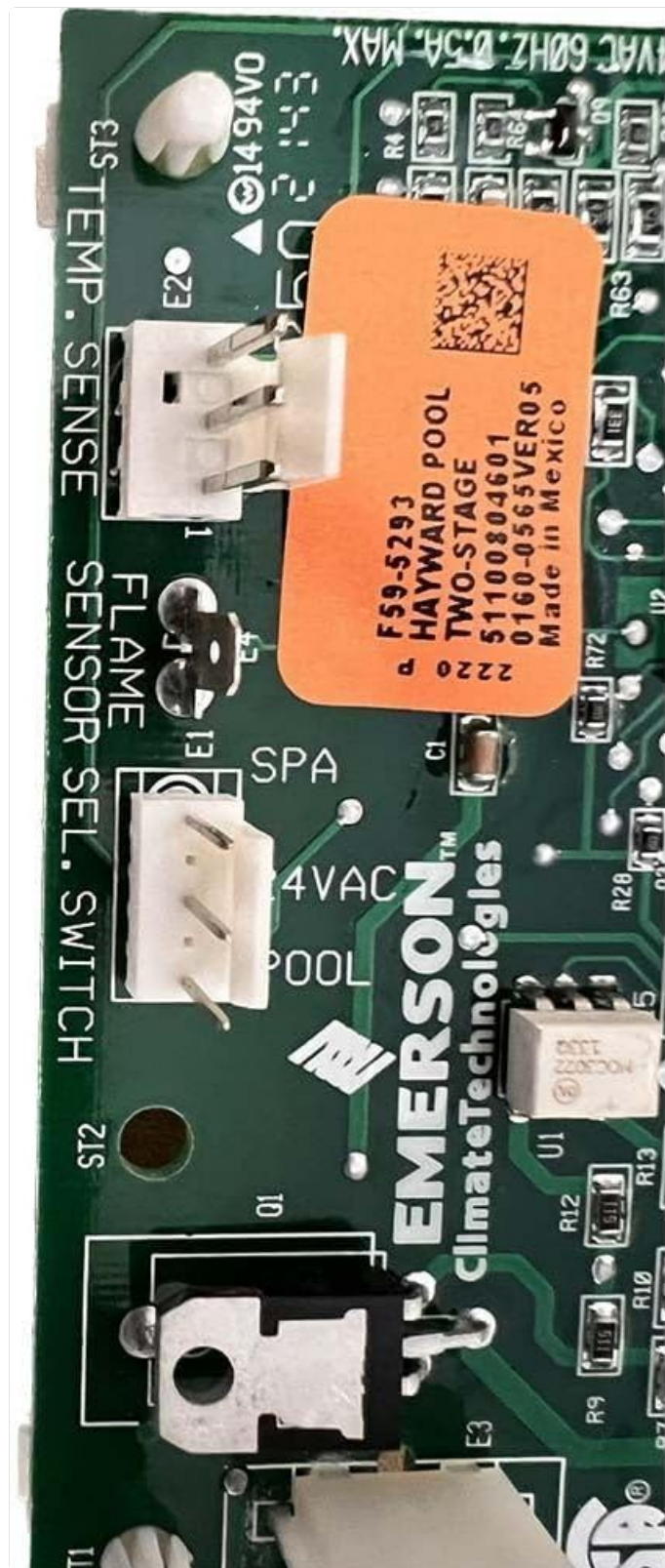
This image provides a detailed view of the sensor and switch connection area on the Hayward HDXFCBRD001 Ignition Control Board. Labels such as 'TEMP. SENSE', 'FLAME SENSOR', and 'SENSOR SEL. SWITCH' are visible, indicating the inputs for temperature and flame detection, crucial for safe and efficient heater operation. An orange sticker with product information is also present.
