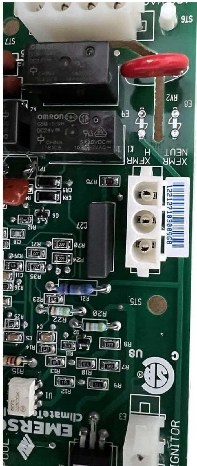
A detailed view of a section of the Hayward HDXFICBRD001 Ignition Control Board, highlighting specific connectors labeled 'XFMR', 'NEUT', 'H' and 'ST5'. A barcode sticker is visible on one of the connectors, likely for identification purposes. This area manages transformer and neutral connections.
