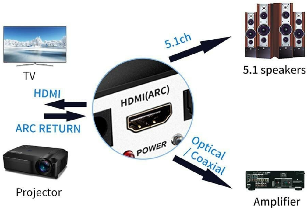
Image 4.2: HDMI ARC connection diagram, detailing how audio is transmitted from a TV or projector to the DA615H for decoding and output to speakers or an amplifier.
