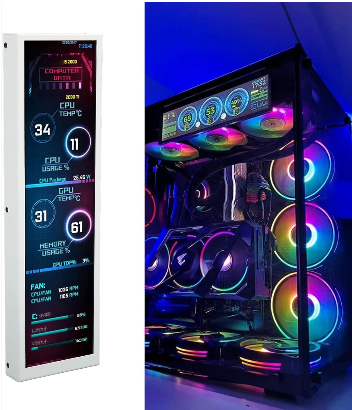
Image: The Dpofirs 8.8-inch Mini PC Sensor Panel Display in a vertical orientation, showing CPU temperature, usage, GPU temperature, memory usage, and fan RPM.
