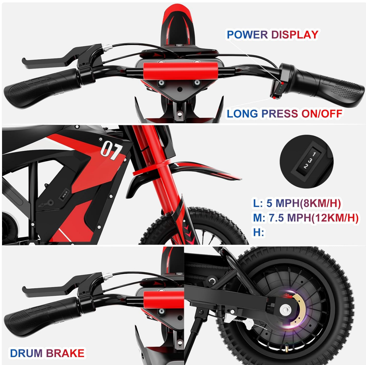
Figure 4.1: Handlebar controls and speed mode selector.
