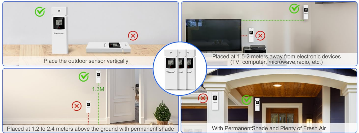
Figure 2: Guidelines for optimal sensor placement, including vertical orientation, distance from electronics, and height for outdoor sensors.
