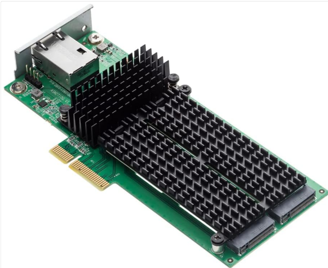
Image: Angled view of the ASUSTOR AS-T10G3 Network Card, highlighting the two M.2 NVMe SSD slots beneath the heatsinks.
