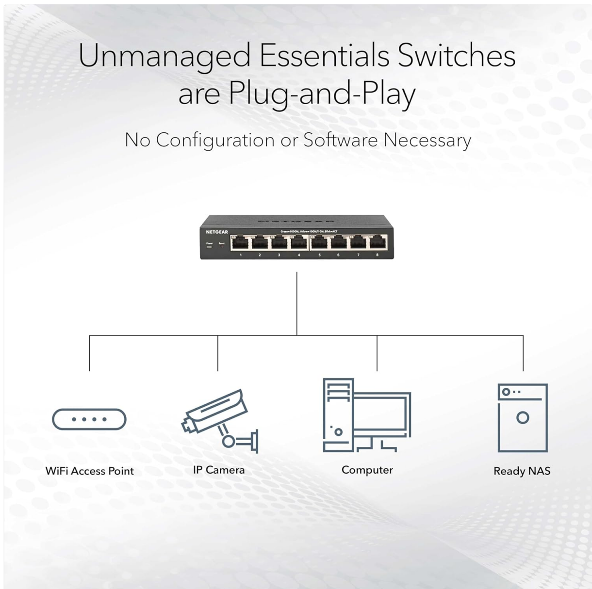
Image: A diagram illustrating the plug-and-play nature of the unmanaged switch, connecting various devices like WiFi Access Points, IP Cameras, Computers, and NAS.
