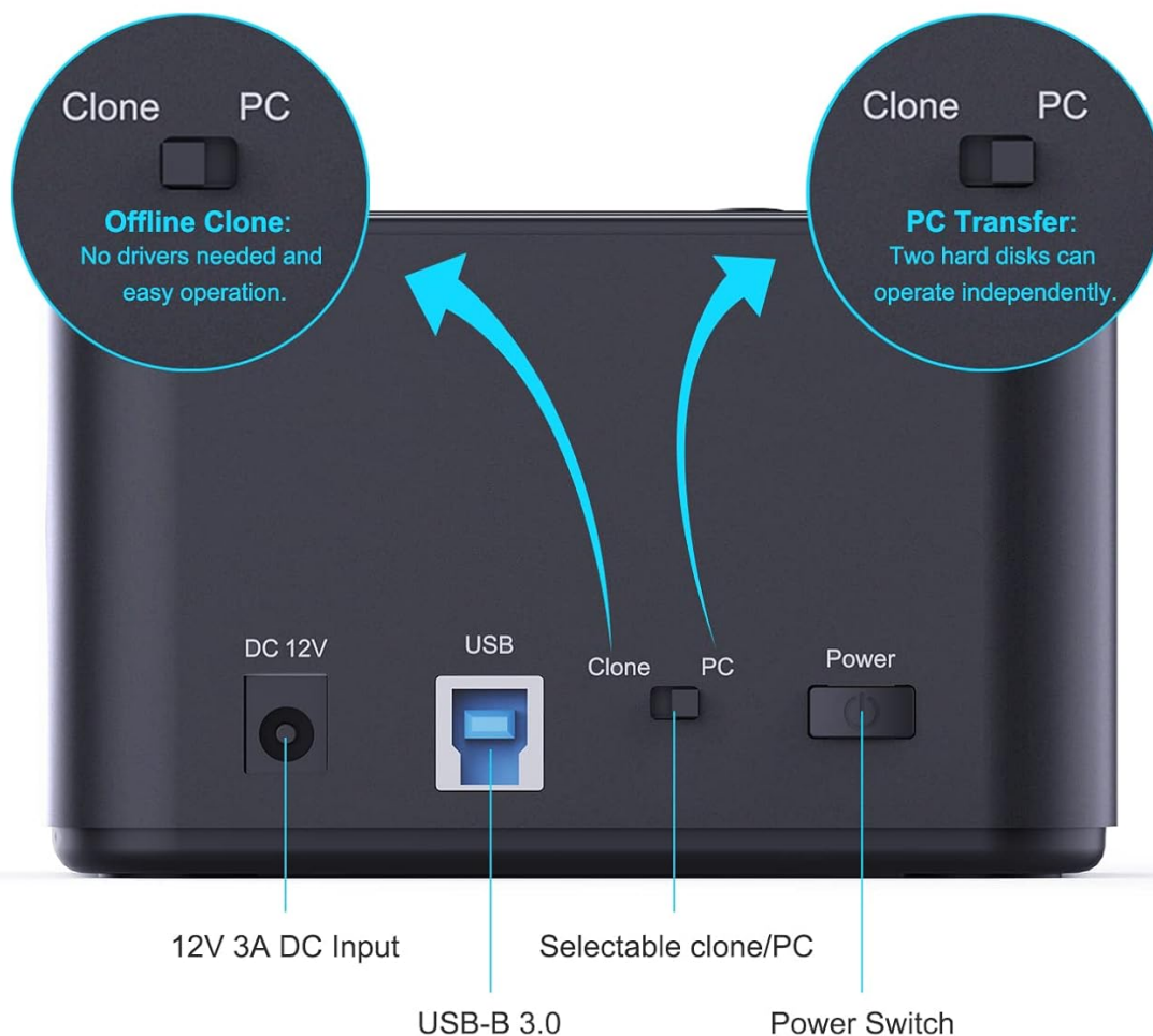
Figure 7: Rear view of the docking station showing the DC 12V input, USB-B 3.0 port, Clone/PC mode switch, and Power switch. The dedicated Clone/PC switch ensures that the desired operation mode is selected, preventing unintended actions.
