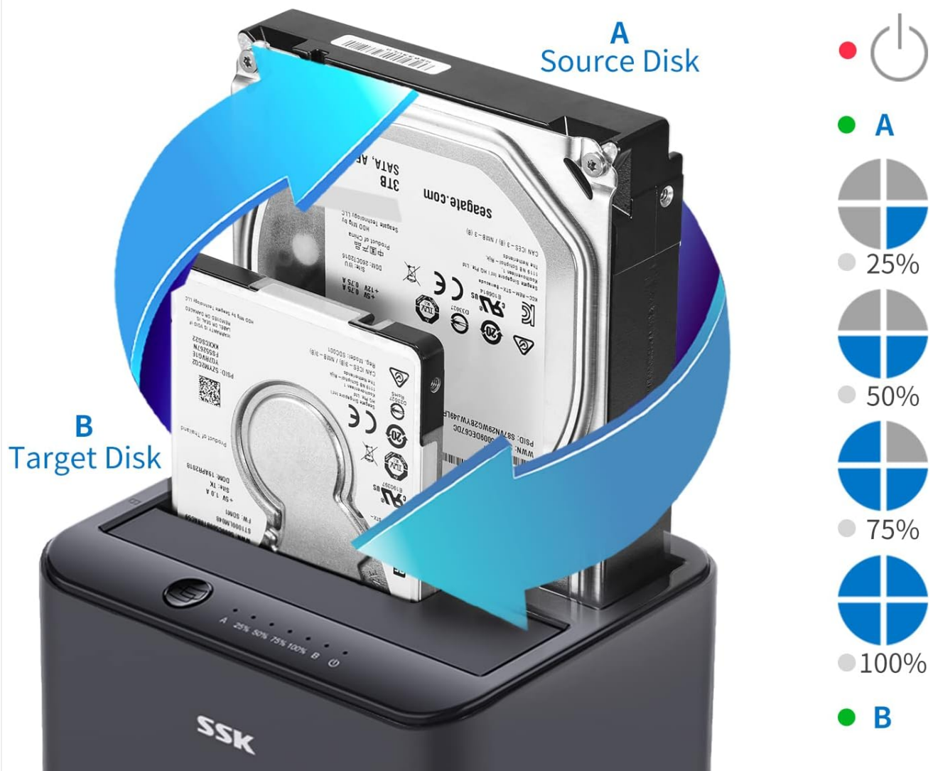
Figure 6: Diagram illustrating the offline cloning process from a source disk (A) to a target disk (B) with LED progress indicators.
