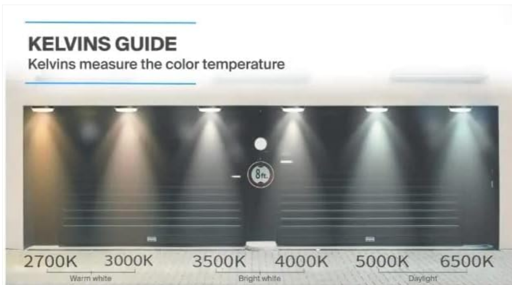
Figure 3: Kelvins Guide. This diagram illustrates different color temperatures (Kelvins) and their corresponding light appearances, from warm white (2700K) to daylight (6500K), helping users understand the tunable CCT feature.
