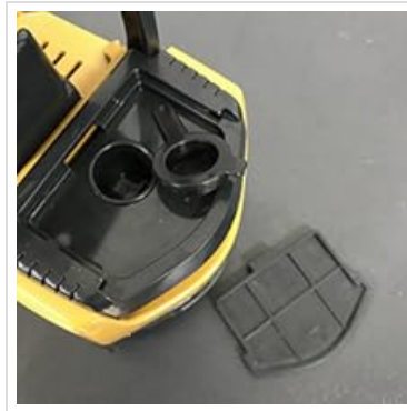
Image: Water inlet for the spray function, located on the top of the forklift.
