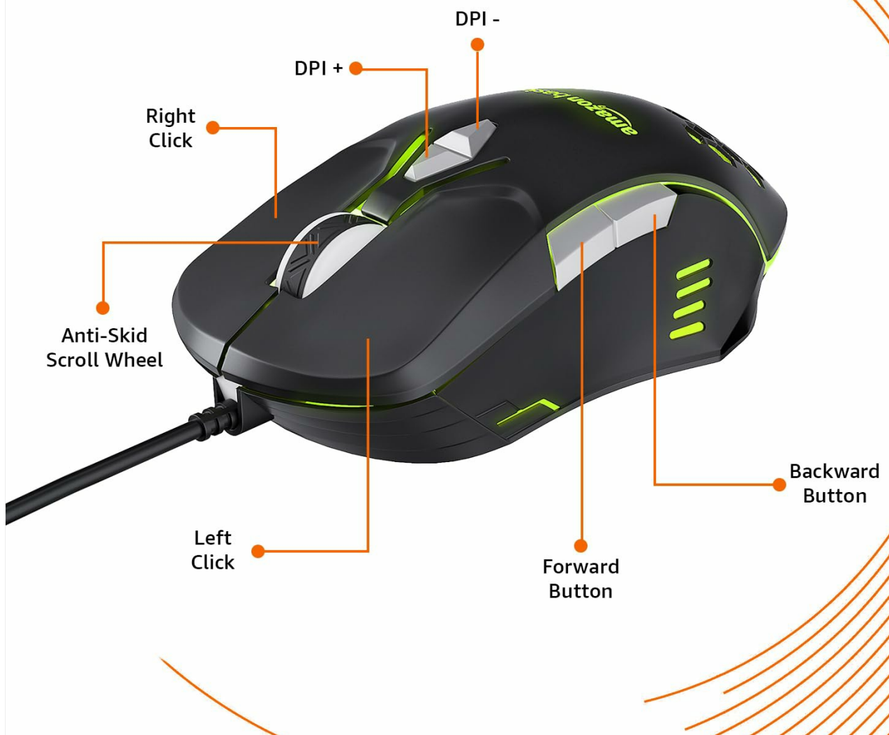
Image: The amazon basics Wired Gaming Mouse showing its 7 pre-programmed buttons, including Left Click, Right Click, Anti-Skid Scroll Wheel, DPI+, DPI-, Forward Button, and Backward Button.
