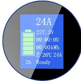
Figure 5.2: The control box allows for real-time data display and adjustment of charging current.
