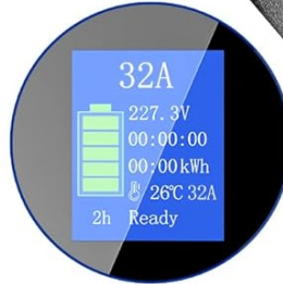
Figure 5.2: The control box allows for real-time data display and adjustment of charging current.
