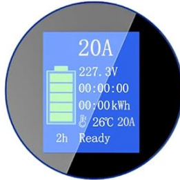
Figure 5.2: The control box allows for real-time data display and adjustment of charging current.
