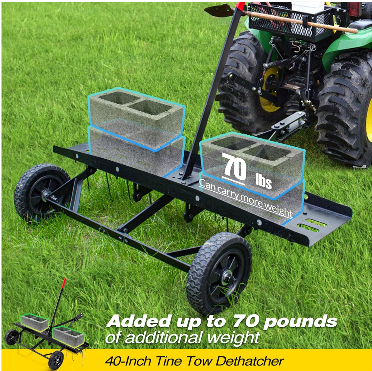
Image: The dethatcher with additional weight on its platform to enhance tine penetration.
