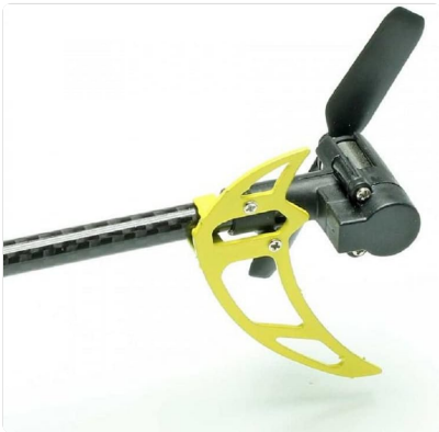
Close-up of the tail rotor assembly, highlighting the yellow fin for visibility. Ensure blades are intact and mechanism is smooth.
